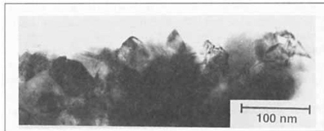
Figure 4. TEM image of the nanocrystalline \text{La}_2\text{NiO}_4 formed by heat treatment at 5°C/min to 950°C.
